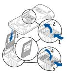
Ensure that the contact area on the card is facing down on the device, and the beveled corner is facing down in the SIM card holder.
