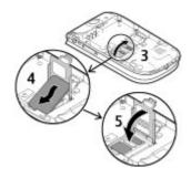
4 Line up the battery contacts, and insert the battery.
