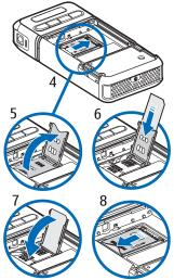
4. Insert the SIM card into the SIM card holder (6). Ensure that
