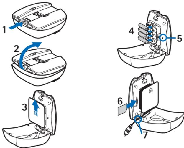
1. Open the main unit by pushing the release bar (1) and lifting the main unit cover (2).
