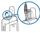
1. Plug the charger transformer into a standard ac outlet.
